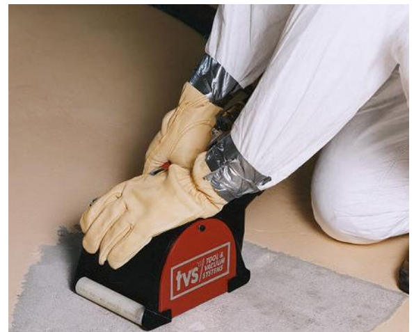
PPT being used in the process of nuclear decommissioning
