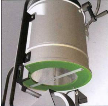
Dust collector filter
